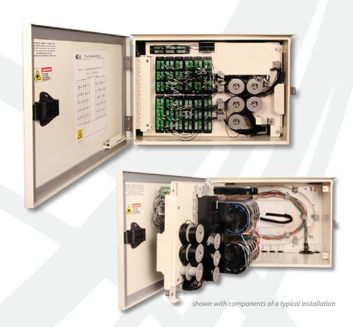
The FDH2 Series is a wall mount fiber distribution hub designed to support patching, splicing and optical splitting in one unit. The enclosure has 13 adapter panel positions allowing for a wide variety of patching and splitting combinations. Two compartments separate the network terminations from the distribution terminations and a single outer door.
